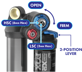
FOX PERFORMANCE ELITE FLOAT X2 Shock Compression Dials
