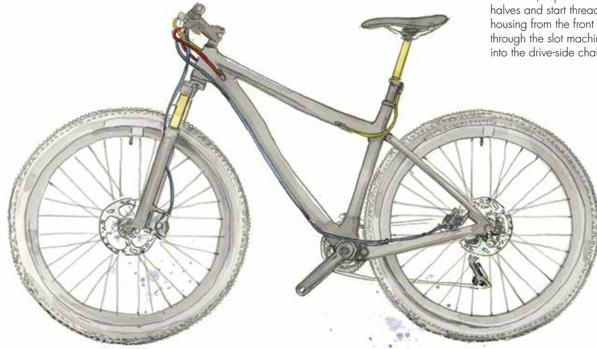
Since we ship the frames with both halves assembled, the person building the bike will have to remove the slot machine hardware, separate the frame halves and start threading housing from the front of the bike, through the slot machine, and into the drive-side chainstay.
